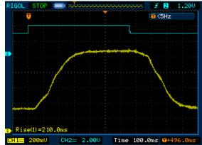
The response of the output (yellow signal) to the unit step of the input signal (blue signal) with the fast filter set. The delay of the output response can be up to 80ms, because this is the period of updating the output signal control by the processor measuring the input signal (with the digital filter set to 0.1s). The rise time resulting from the analog time constant is about 200ms. The total time of setting the output can be about 200...300ms.
