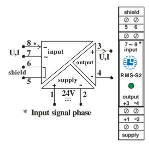
**Note:** Terminals 5-6 are used to connect the braided shield of the input signal cable. If the input signal (terminals 7-8) is not galvanically separated from the ground GND or PE terminals 5-6 (shield) cannot be connected to GND or PE. Terminals 5-6 can be connected to the braided shield of the input signal cable only if the braided shield is not connected to the ground GND or PE from the other side of this cable.
